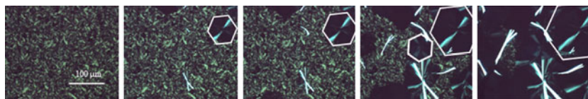
Fig. 14 Sequence of different pictures taken at intermediate temperatures starting at the ILC phase (at the left ), and ending at the SI (rotator phase), showing the hexagonal growth of this phase
